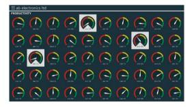
This dashboard is displaying gauges for KPI's and actual machines line status. The 5 production lines are demonstrating the wide range of machine brands available.
